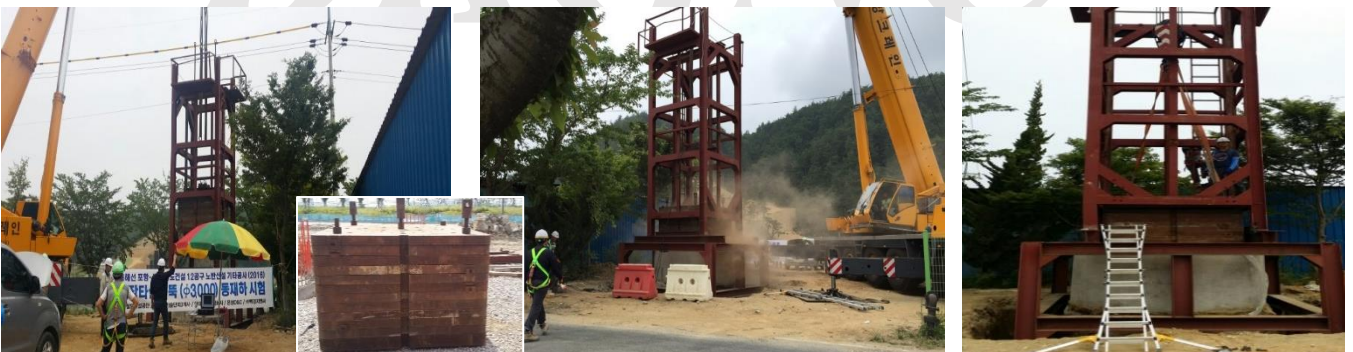
PDA Test for Drilled Shaft pile : Drop ram weight (39.1ton)
