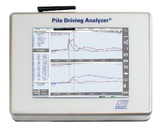
PDA Test for Drilled Shaft pile : Drop ram weight (39.1ton)
